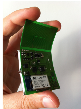
Fig. 1. Photo of the IronIC Patch. The system can be placed over the implantation area to power implanted sensors and communicate with them.
