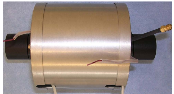
Figure 7. Fully assembled resonator package with 25 mm diameter cell.
