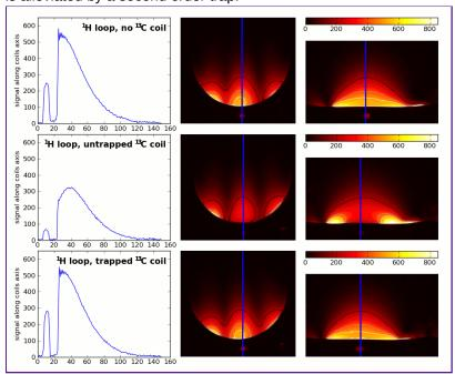
Adding the second order trap has only minor impact on 13C SNR (<5% as line width corrected comparison of peak height/noise, and <1% when SNR is determined from an AMARES fit.)
