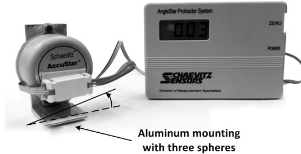
Figure 6.31: Schaevitz Sensors AccuStar inclinometer (Measurement Specialities TM [56], \pm 20^\circ stroke, 0.01^\circ resolution); the mounting including three spheres allows to precisely position the measurement device on the robot output. [54]
