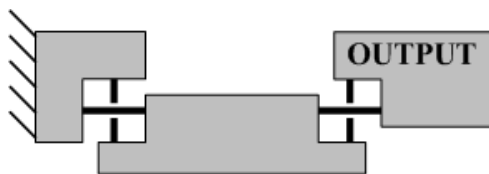
Figure 5.20: Sketch of a t_{\parallel}r_{\perp} , t_{\perp}r_{\parallel} and t_{\parallel 1}r_{\parallel 2} bricks design solution, featuring two separated crossed-blades pivots
