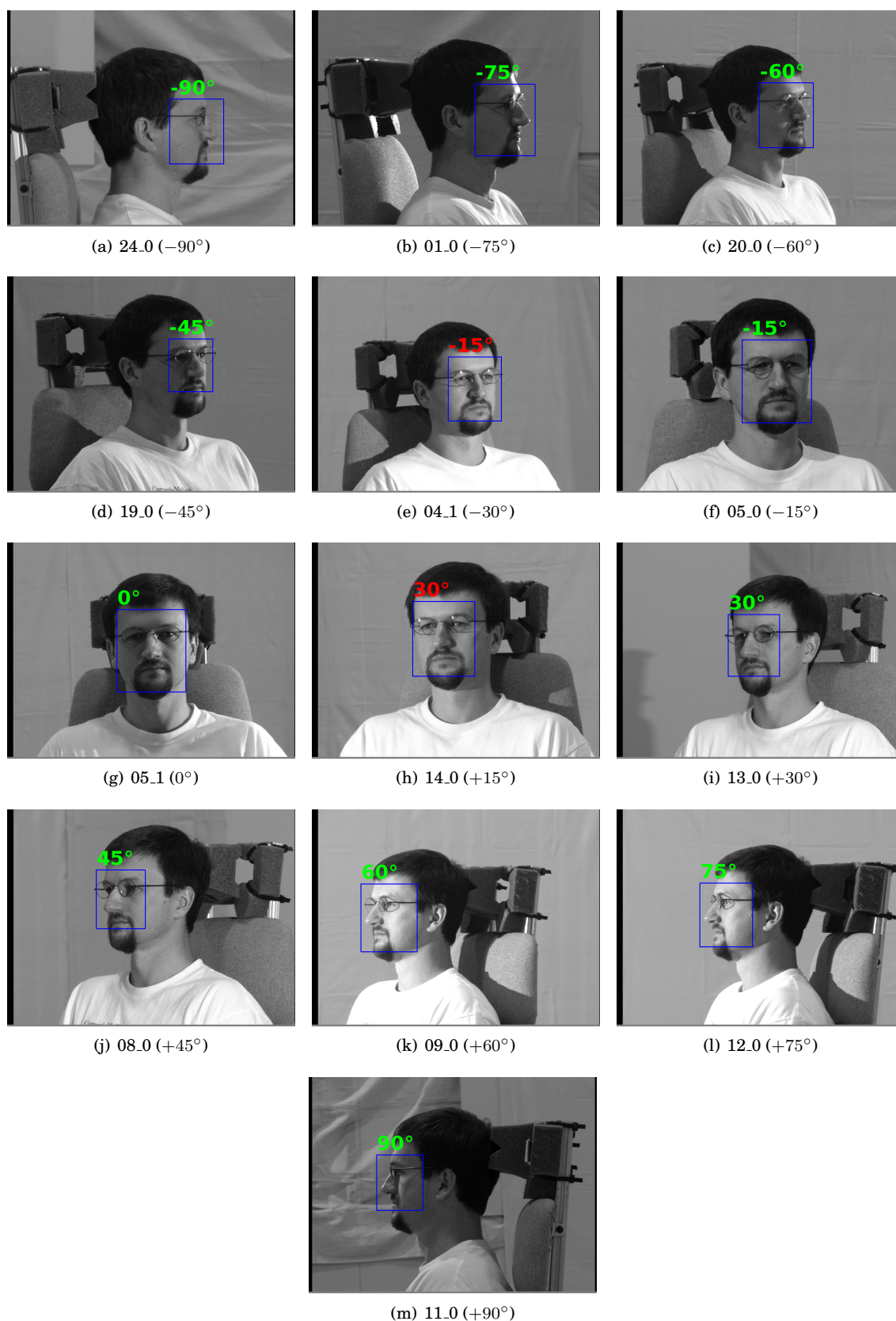
Figure 7.4. Illustration of some face pose classification results on the CMU MultiPIE test dataset: from right profile (a) to left profile (m). The face bounding box is represented with the blue rectangle. The classified poses are displayed in angles with green if correct and with red if incorrect respectively.
