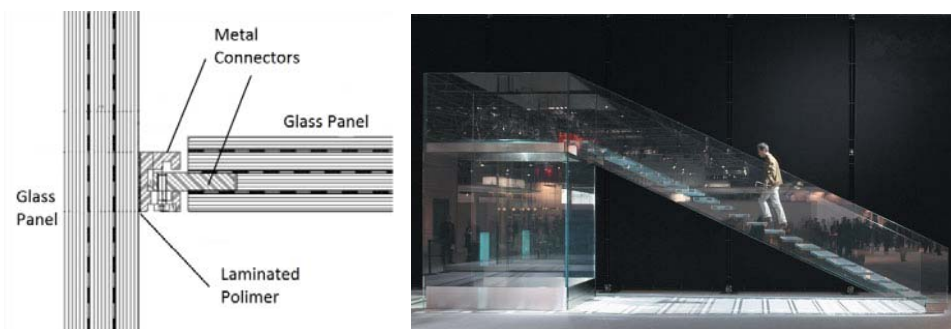
Figure 3. Real scale application of laminated connection in structural elements.(See staircase) [22]
