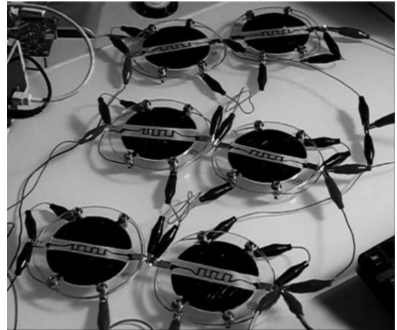
Fig. 4. Ring oscillator during oscillation. Three inverters are connected in a ring (bottom → middle → top) and when powered will oscillate.
