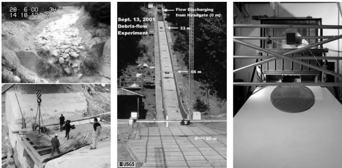
Figure 1.4: Different research scales. Left: In situ observation in the Illgraben: Instrumentation of the bed with a force plate and pore pressure sensors [21]. Center: Large-scale experiments into the USGS Debris-flow flume [17]. Right: Laboratory idealized experiments: dam-break of Carbopol gel on an inclined plane, measurement of the free surface topography [22].
