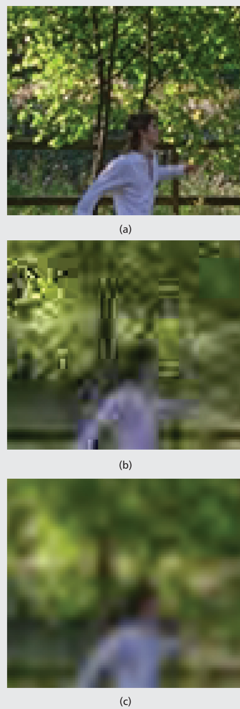
Figure 2. Example of visual distortions resulting from different combinations of scalability options for scalable video coding (SVC), the scalable extension of the latest H.264/AVC: a) the original video frame; b) blockiness in the video frame encoded with SVC at a low bit rate; c) blurring in the video frame encoded with SVC at 1/16 of the original resolution and upsampled to the original resolution for presentation to the user.
