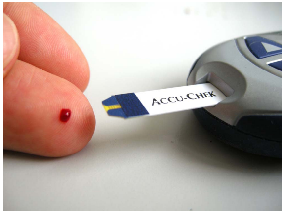
Figure 1.2: Procedure for self-monitoring of blood glucose: a drop of blood is applied on a test strip inserted on a handheld glucose meter.
