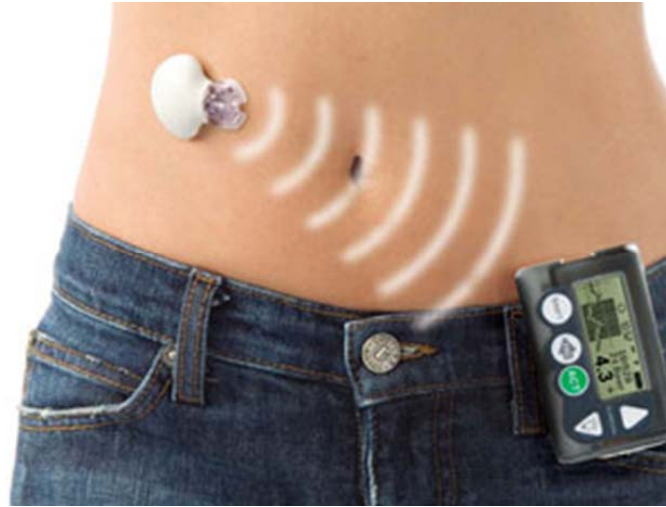
Figure 1.4: Example of commercially available subcutaneous implantable needle-type glucose sensor (Guardian REAL-Time System from Medtronic).
