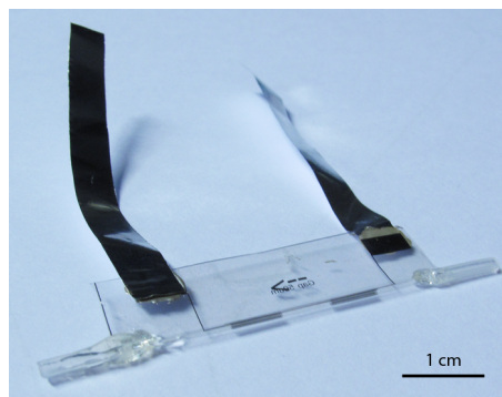
Figure 7.3: All-around-electrode ACEO micropumps fabricated by lift-off of Cr/Pt electrodes on thin PET foils, which were folded and bonded following the described procedure.
