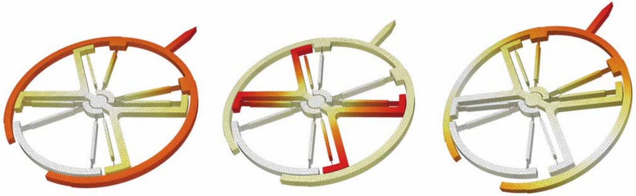
Figure 2: SolidWorks finite element modal analysis of the rotor's mechanical structure. The color levels describe the displacement magnitude relative to the anchor. From left to right, we show the first eigenmodes occurring at 170 Hz, 683 Hz and 2810 Hz, respectively. The first mode corresponds to the in-plane vibration of the rotor ring, while the second mode corresponds to the in-plane vibration of the internal butterfly pivot.
