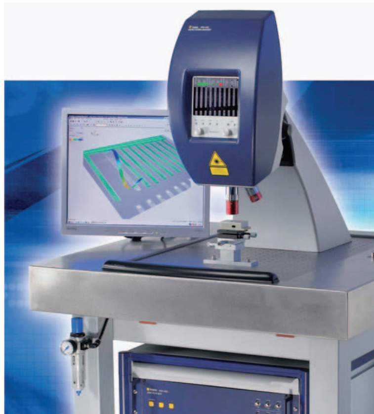
Figure 4.1: Polytec MSA-400: All-in-one state-of-the-art instrument dedicated to MEMS and microstructures' analysis. Figure reproduced from [8].
