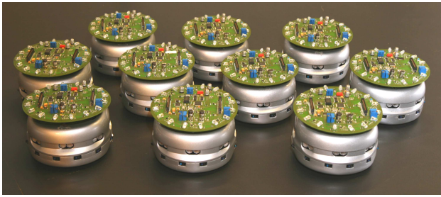
Fig. 3. Fleet of ten Khepera III robots. The robots are all equipped with an inter-robot, relative range and bearing module, which is composed of a ring of 16 infrared LEDs.
