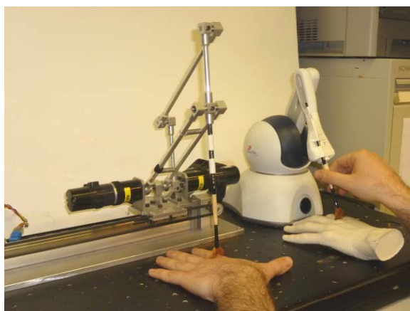
Fig. 5. Experimental environment. The master device (PHANTOM Omni) and the slave device are located in front of the blindfolded participants' right and left hands, respectively. The participants manipulate a paintbrush attached on the master device to brush the rubber hand, which was located 200 mm right from the participant's left hand, in their own way. The slave device synchronously or asynchronously gives the same brushing on the participants' own hand.
