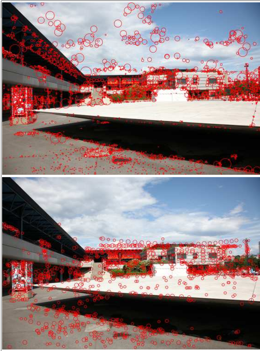
Fig. 1. Keypoint detections by DoG (top) and our proposed detector TaSK (bottom). Note that TaSK is specialized to focus more on stable man-made structures and ignores vegetation and sky features.
