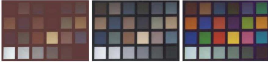
Fig. 5. Raw image of the projected digital GretagMacbeth color chart (left); outcome of the linearization and dark frame removal step (middle); result after subsequent color transformation (right).
