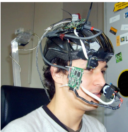
Figure 2: A portable eye-gaze tracker mounted on bicycle helmet monitors the user's attention patterns helping us to quantify the effects of the collaborative control system on the user's perception [12].
