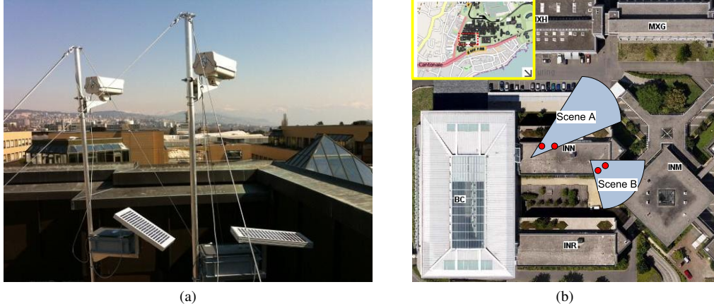
Fig. 4. Experimental setup to capture datasets: (a) Two surveillance cameras with solar power system watching Scene B. (b) The setup of two cameras (red dots) on roof of a building in campus. Scene A and B show the viewpoints of two datasets.
