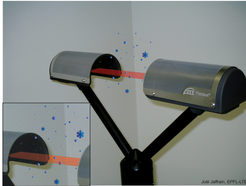
Figure 2.1: The optical disdrometer Parsivel® (OTT). The measuring principle is based on laser attenuation when a particle crosses the beam.
