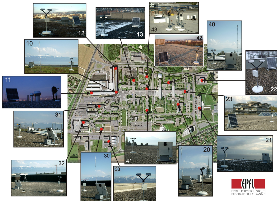
Figure 2.3: The network of 16 Parsivels deployed over EPFL campus ( \sim 1 \times 1 \text{ km}^2 ) in Lausanne, Switzerland.
