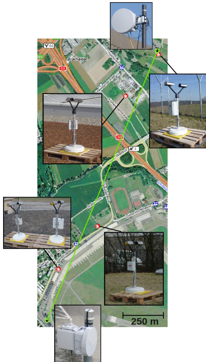
Figure 6.5: The COMMON field campaign involves a microwave link deployed over a 1.85 km distance, 5 autonomous disdrometers deployed at 4 sampling locations and 3 tipping bucket rain gauges (courtesy of Marc Schleiss, EPFL-LTE).
