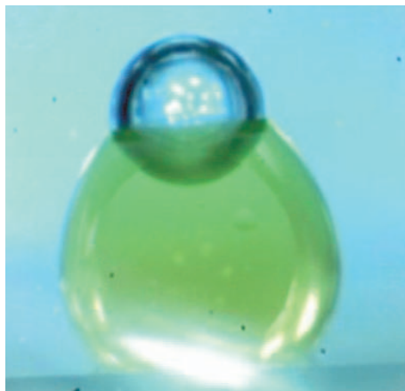
Fig. 4. \text{H}_2 bubble forming on a 1,2-DCE droplet containing DMFc in an aqueous HCl (pH = 1) solution.
