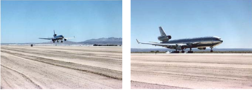
Fig. 2.11 Landing demonstration of MD-11 Propulsion Controlled Aircraft (PCA), NASA Dryden, 2001 (copyright NASA)
