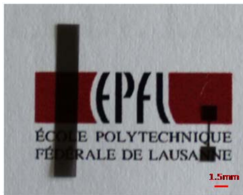
Figure 6.12: Rectangular and dog-bone structures lifted-off from the wafer after photo-patterning.
