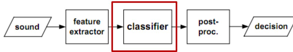
Figure 1: Basic structure of a sound classification system comprising feature extraction, classification, and postprocessing.
