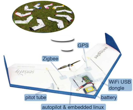
Fig. 3. Aerial swarm composed of 10 flying-wing robots.
