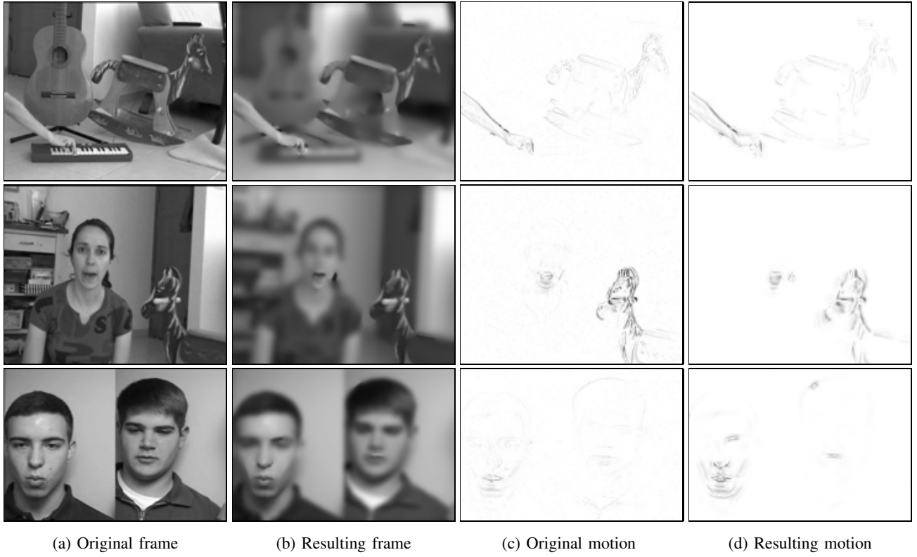
Fig. 7. Results obtained when applying our method to MovieA , MovieB and MovieC with K = 0.1 . The diffusion process has been automatically stopped after n_{stop} = 26, 25, 11 iterations respectively according to the stopping criterion in Sec. III-B.
