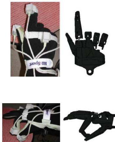
Figure 2.18: An example mapping of a human pointing grasp using the Robonaut Hand [EK04].
