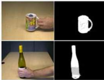
Figure 2.25: Handle-graspable Vs sidewall-graspable objects. Interaction regions are given in grey [SLZS08].
