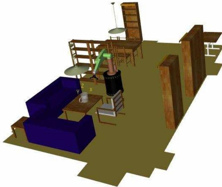
Figure 6.1: Grasping the mug by its handle is impossible in such situation (This is a GraspIT environment [MKAC03]). Another grasp should thus be computed.
