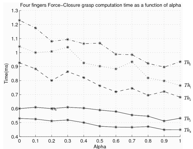
Fig. 4. 4-finger force-closure grasp computation time using our method with thresholds Th0 < Th1 < Th2 < Th3 < Th4
