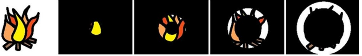
Figure 1: An example of circular segmentation and concentric cropping of an image into 4 concentric regions.
