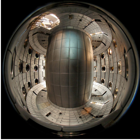
Figure 1.8: Internal view of the TCV tokamak (Lausanne, CH. R_0 = 0.88\text{m} , a = 0.25\text{m} ). Note the large number of ports and protective carbon tiles. This photo was taken just after the tiles had been cleaned.
