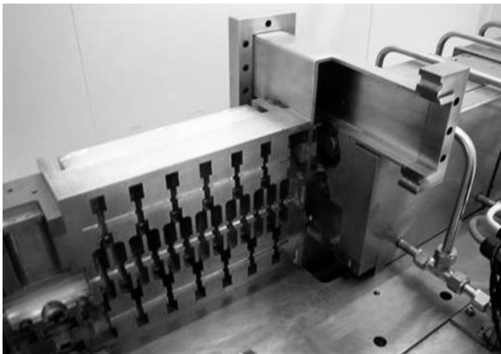
Figure 2.4: Cut section of the prototype of LIBO (courtesy of TERA)
