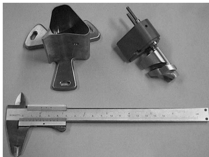
Figure 5.8: Photograph of the K800 (LNS) spiral inflector electrodes and housing[Rifuggiato and Calabretta, 2000]. Note that \rho_m \simeq 1.123 cm, \rho_e \simeq 2.7 cm and K \simeq 1.2
