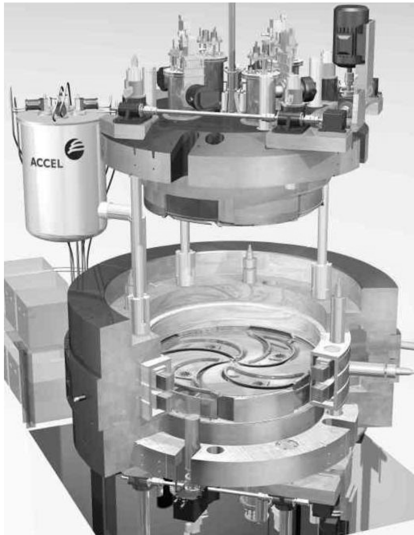
Figure 2.3: Model cut view of COMET with lifted upper pole cap
