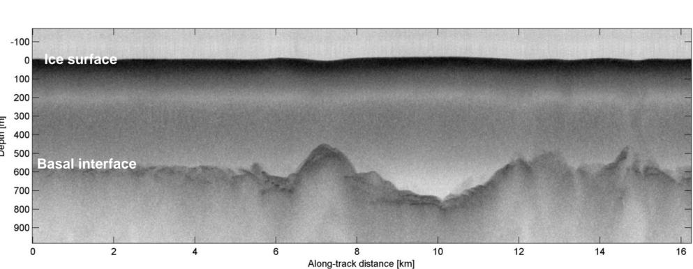
The floating tongue of the Jutulstraumen Glacier is seen in the middle of the profile. Four separate apertures are combined coherently (not yet any clutter suppression).
