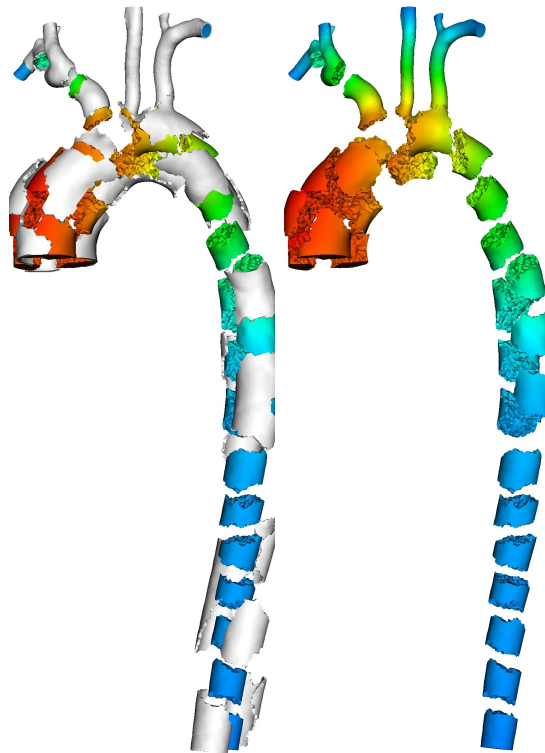
Figure 5.18: Aorta mesh partitioned with 32 processors using ParMETIS. The mesh is composed of 380'690 tetrahedra, i.e., 486'749 dofs.. On the right: the fluid mesh partitioned; on the left: both fluid and solid mesh partitioned.
