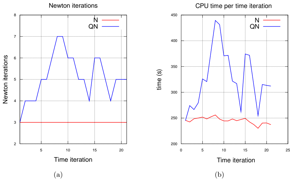
Figure 5.38: Aorta simulation: (a) number of Newton iterations and (b) CPU time per time step. Exact Newton (N) is compared versus inexact Newton (QN) for an interval during the systolic peak (from t = 0.16 s to t = 0.24 s) for a GI simulation with time step \delta t = 0.004 s
