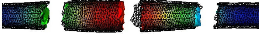
Figure 6.1: The cylindrical geometry used partitioned into 4 subdomains. One processor holds one solid and one fluid subdomain. However, in general, the two are not matching on the interface (despite the impression given by the picture) and the partitioning is done independently for the two meshes.
