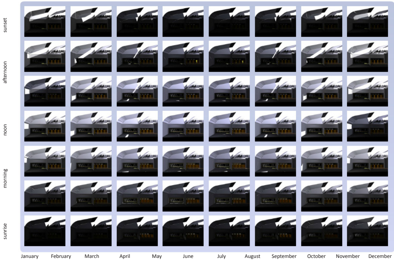
Top: view towards east facing windows during early afternoon in late fall, top view during afternoon in early spring, windows during early afternoon in late fall Bottom: time-varied renderings of view towards east facing windows under intermediate sky conditions
