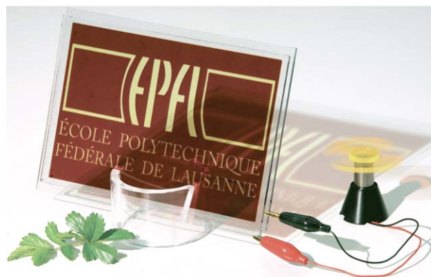
Fig. 2 (Top) Operating principles and energy level diagram of dye-sensitized solar cell. S^{\circ}/S^+/S^* = sensitizer in the ground, oxidized and excited state, respectively. Red/Ox = Redox mediator. (Bottom) Example of a DSC (Ecole Polytechnique Fédérale de Lausanne).
