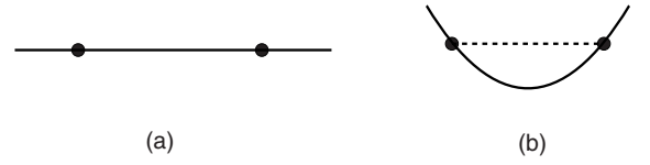
Fig. 7. Schematic representation of why inextensibility constraints are ill-suited for sharp folds. (a) Two points of the discrete representation of a continuous surface in its rest configuration. (b) When deformed, while the geodesic distance between the two points is preserved, the euclidean distance decreases. This suggests that distance inequality constraints should be used rather than equalities.
