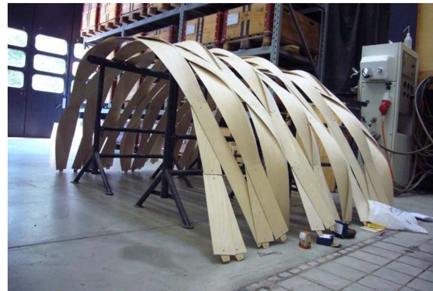
Timberfabric, interconnected elements, continuity in two directions;
