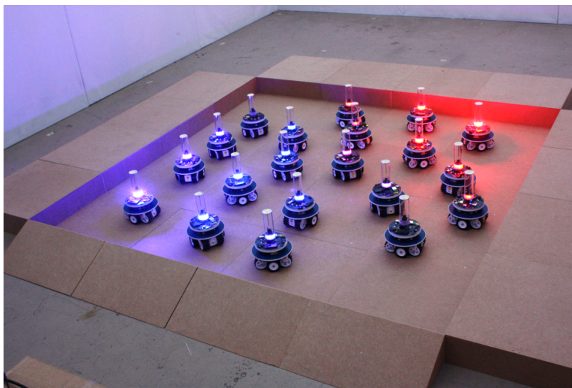
Fig. 10 Example of arena configuration with twenty marXbot robots.
