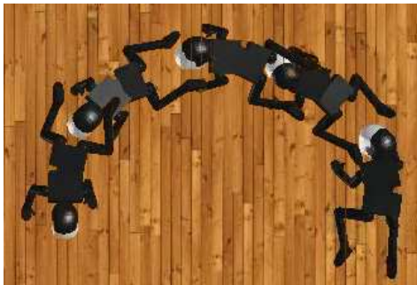
Figure 23: The iCub turning. Superimposed snapshots of the robot turning with a torso angle of 0.5 radians. Movie available as Online Resource, Movie 6.
