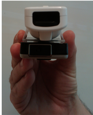
Fig. 6. Drag-and-drop remote control with pico projector
