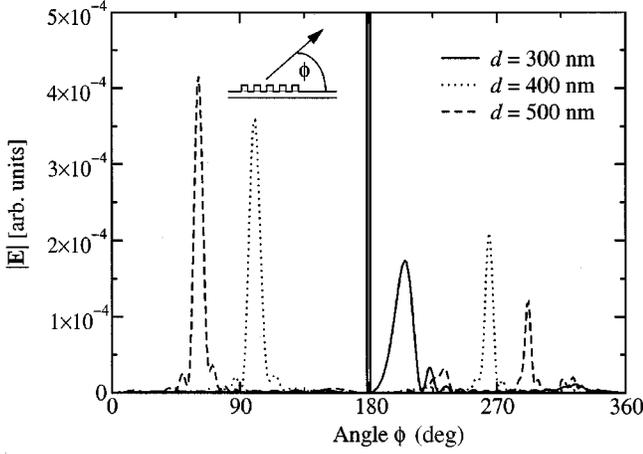
FIG. 7. Angular distribution of the electric-field amplitude  $50 \mu\text{m}$  away from the center of the three gratings in Fig. 6. The central peak at  $\phi = 180^\circ$  is caused by the mode in the guiding Si layer and appears also at  $\phi = 0^\circ$  and  $\phi = 360^\circ$  (not shown).
