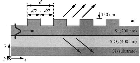
FIG. 5. Geometry of the SOI planar waveguide (permittivities  $\epsilon_{\text{Si}}=12.3$ ,  $\epsilon_{\text{SiO}_2}=2.1$ ; wavelength  $\lambda=1.3$   $\mu\text{m}$ ). A Si grating with 150-nm height, periodicity  $d$ , and a 0.5 filling factor is etched on top of the waveguide.
