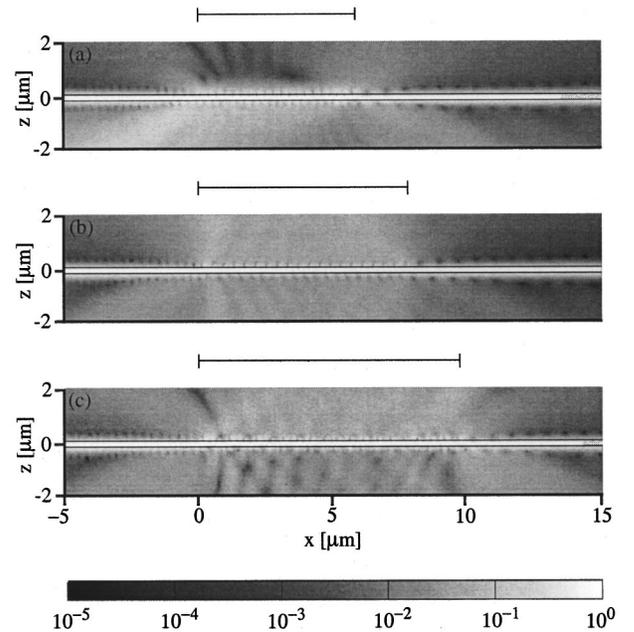
FIG. 6. Electric-field amplitude in the structure of Fig. 5 with three grating periodicities: (a)  $d=300$  nm, (b)  $d=400$  nm, and (c)  $d=500$  nm. The bars represent the total length of each grating. The systems are illuminated with a  $\text{TE}_0$  mode propagating in the  $x$  direction. For clarity, the guiding silicon layer is marked with two lines. A logarithmic color scale is used.
