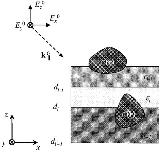
FIG. 2. Projection of Fig. 1 on the  $xz$  plane. This plane is normal to the direction of translation symmetry and the investigation of the system can be restricted to this plane. Note that only the projection  $\mathbf{k}_{||}^0$  of the incident wave vector  $\mathbf{k}^0$  is shown and in general all three components of the incident electric field are nonzero.
