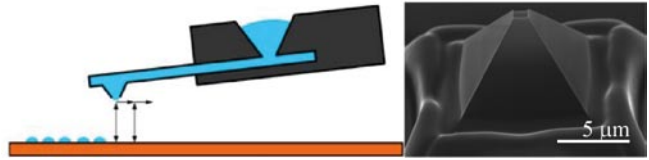
Fig. 3. Conceptual drawing of the nanodispenser and SEM image of a modified tip
