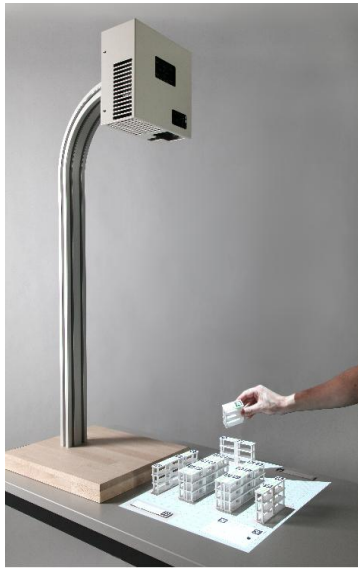
Figure 1a. Students construct and run simulations of a warehouse model built with tangible objects (shelves, docks, etc.)
