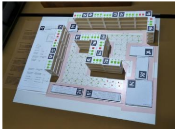
Figure 1b. A camera and a projector enable visual feedback to be augmented directly on top of the physical model.
