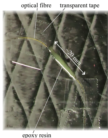
Figure 2.8: Photo of surface-glued optical fibre.
