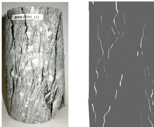
Figure 6-12: Comparison of laboratory compressive failure of Augig granite with CFM predictions under unconfined condition
