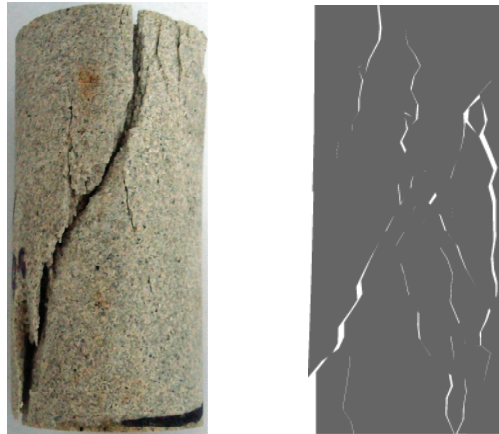
Figure 6–23: Comparison of experimental compressive failure of Transjurane sandstone with CFM predictions under unconfined condition
