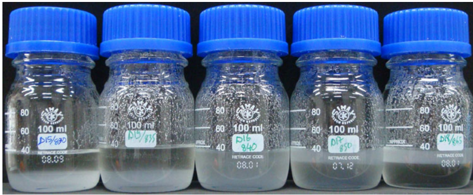
Fig. 7 The 1-week sedimentation experiment: from left to right, fluid densities of 1.1830; 1.1835; 1.1840; 1.1850; and 1.1865 \text{g}/\text{cm}^3 . The bright part results from a concentration of particles while the dark part means that the corresponding local volume is almost free of particles.
