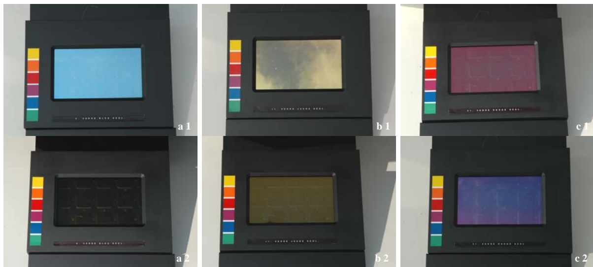
Fig.4: Demonstration box showing the effect of sun (up) and shadow (down) on different colour samples: a1-a2: blue coating; b1-b2: yellow coating; c1-c2: red coating
