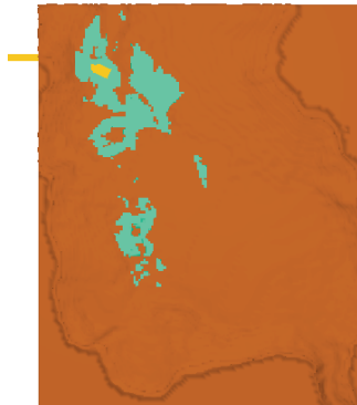
Figure 9 : Suspended sediments in the Räterichsboden Reservoir while turbidity currents entering the Reservoir [t=500 sec]
