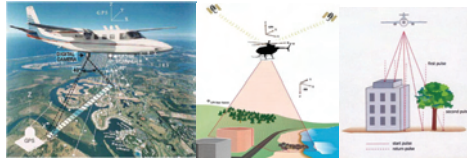
Figure 10, Système LIDAR(Light Detection And Ranging)
