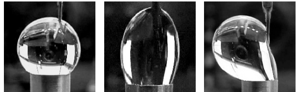
FIG. 5: Left: ideal spherical drop (3.5 ml), Center: attracted oblong drop (7 ml), Right: repulsed drop (5 ml).
