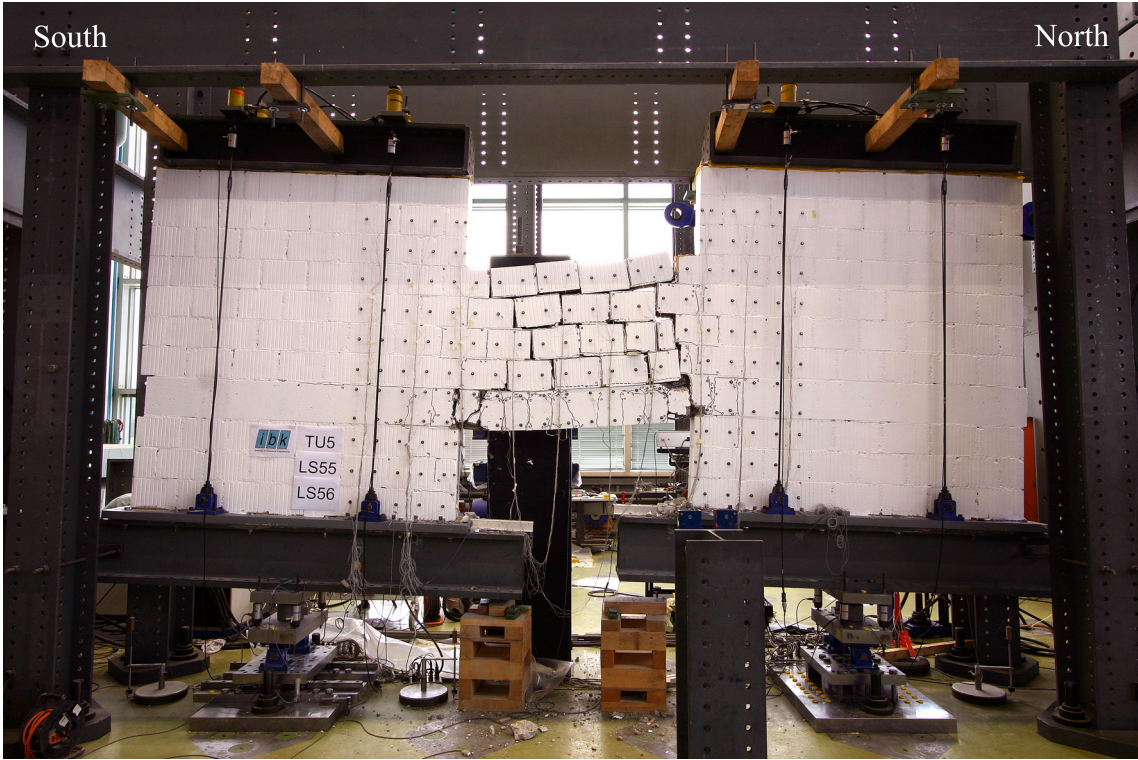
Figure 3.56: TU5: Test unit at LS 56. Drift towards North with \theta_{nom} = 4\% (failure of TU5).
