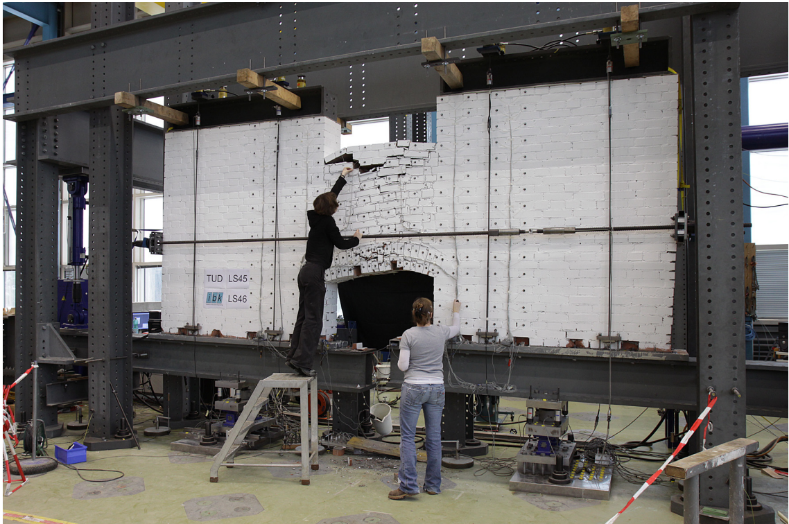
Figure 1.12: Photo of the test setup for the masonry spandrels with arch (TUC and TUD). View from the East during testing of TUD.
