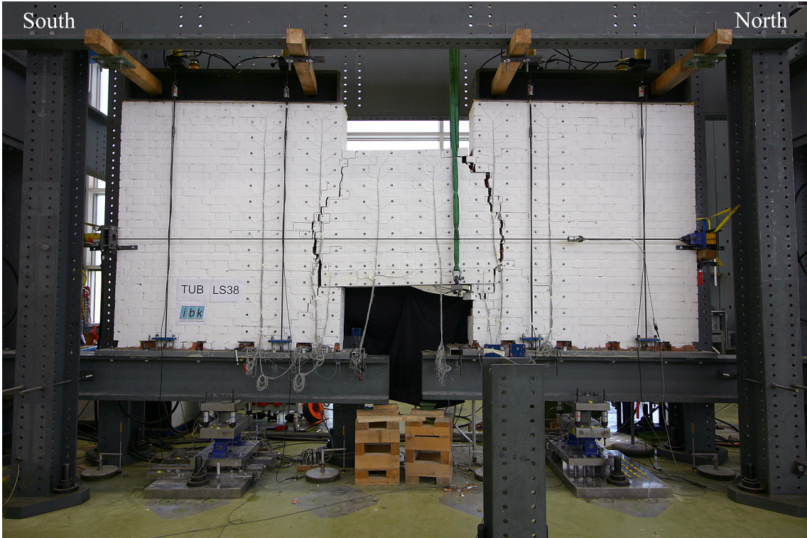
Figure 3.19: TUB: Crack pattern of spandrel at LS 38. Drift towards North with \theta_{nom} = 1.5\% .
