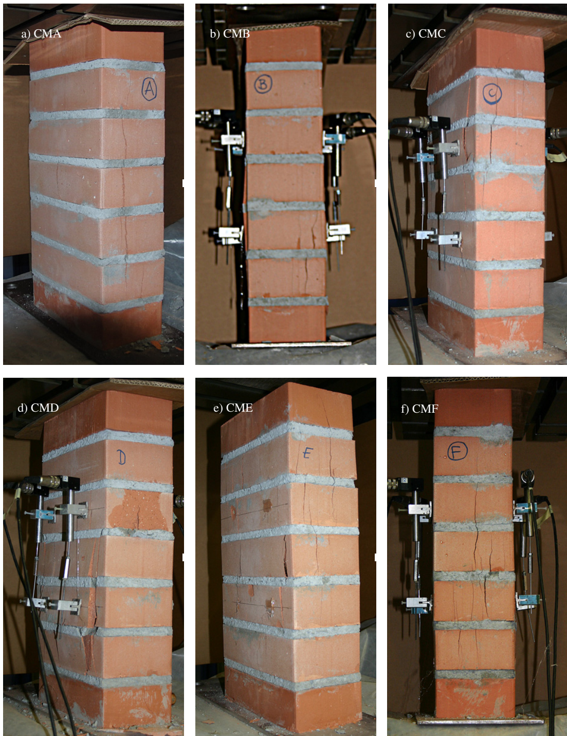
Figure 2.15: Compression tests on masonry wallettes: Crack pattern after failure for units CMA-CMF.
