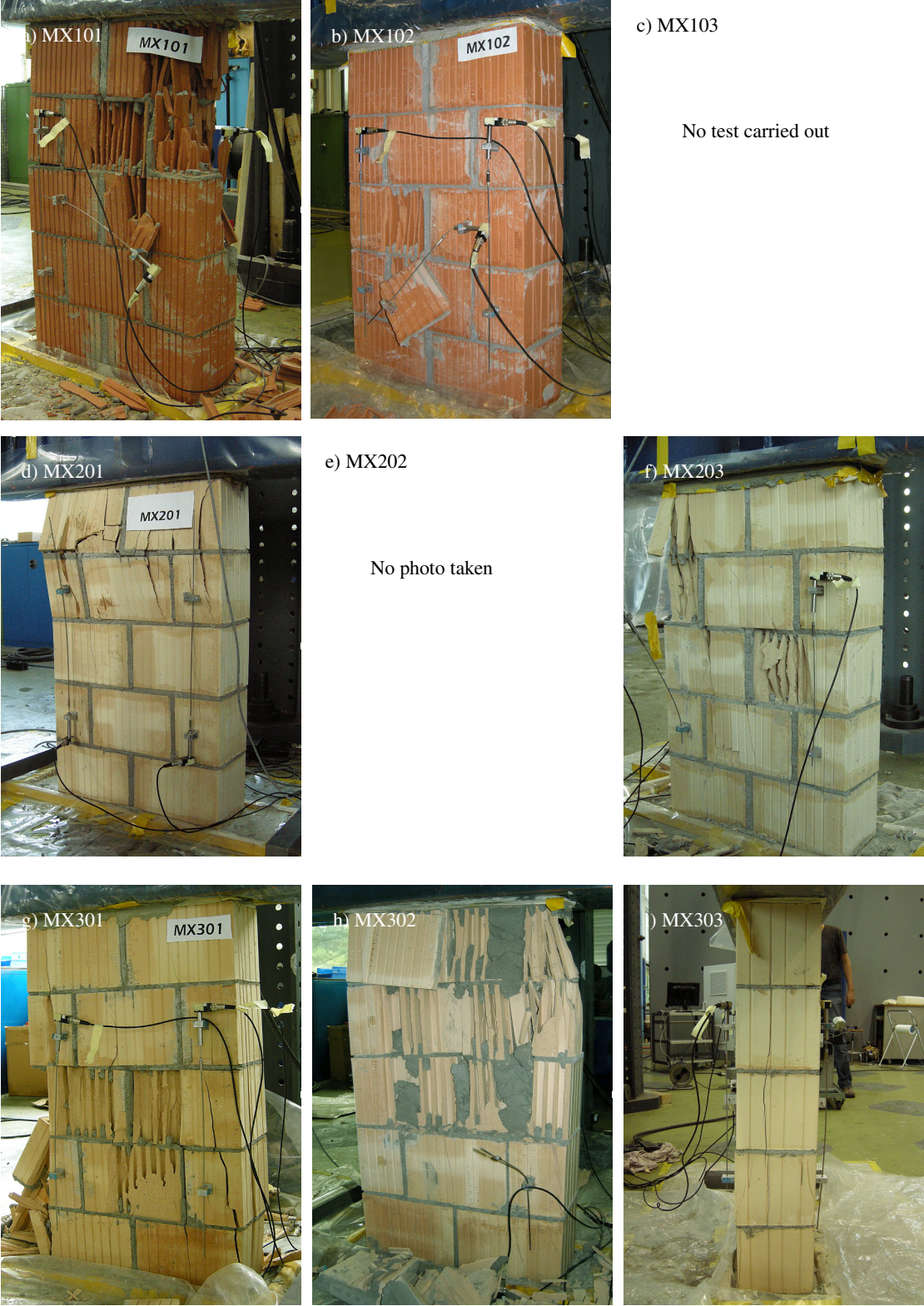
Figure 2.14: Failure modes of masonry wallets tested under compression orthogonal to the bed joints.
