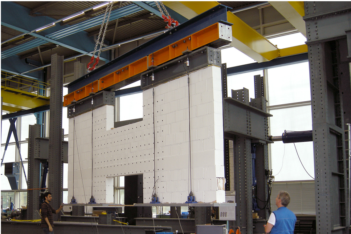
Figure 1.4: Lifting the test unit onto the test stand.
