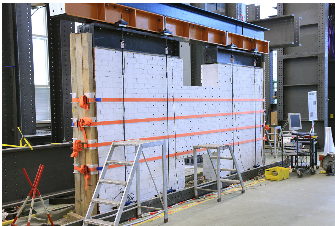
Figure 1.5: Test unit ready to be lifted onto the test stand.
