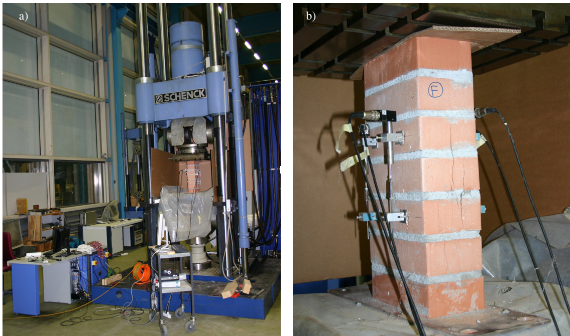
Figure 2.12: Compression tests on masonry wallettes: Global view of the test setup (a) and detail of a wallette with the instrumentation (b).
