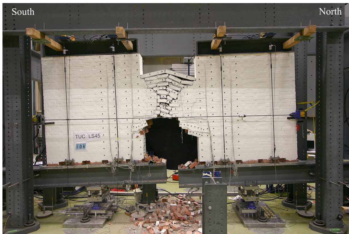
Figure 3.34: TUC: Crack pattern of spandrel at LS 45. Drift towards South with \theta = -3.5\% (failure of TUC, \theta_{nom} = -2.0\% ).
