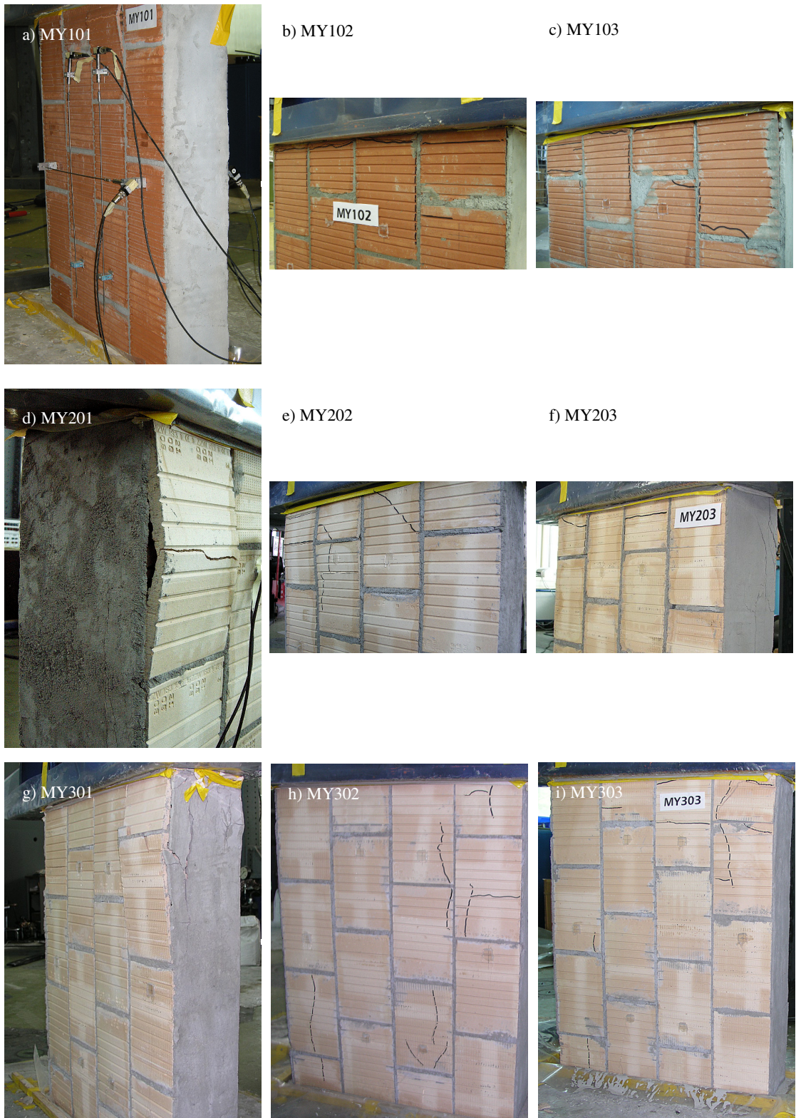
Figure 2.15: Failure modes of masonry wallettes tested under compression parallel to the bed joints.
