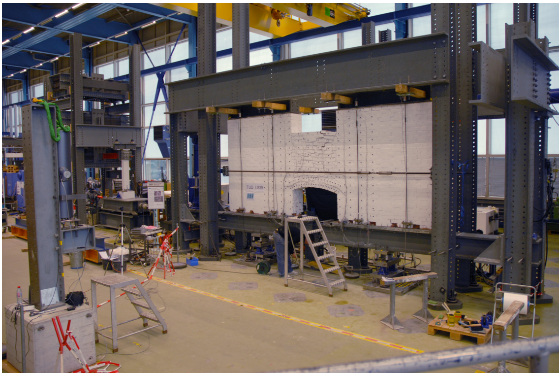
Figure 1.17: Test setup including Optotrak position sensor. View from the North-East.
