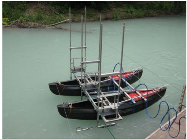
Figure 2: Array of Nortek Acoustic Doppler Velocimeters (ADV) in the field investigations.
